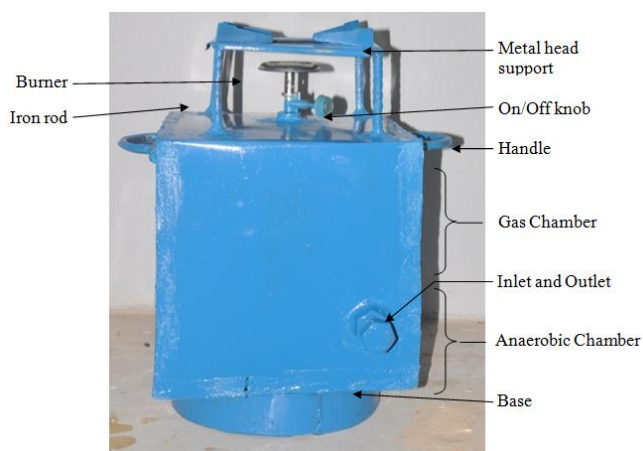
Plate 1: Biogas production design for rural communities
